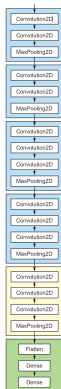
The VGG-16 CNN model (F. Chollet: Deep learning v jazyku Python, obr. 8.15)
