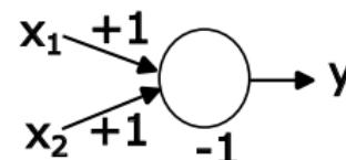
$$\begin{aligned}y &= \text{sign}(w_0 + w_1 x_1 + w_2 x_2) \\&= \text{sign}(-1 + x_1 + x_2)\end{aligned}$$
