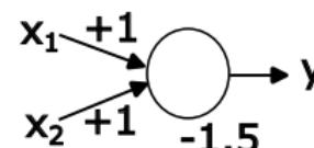
$$\begin{aligned}y &= b\text{sign}(w_0 + w_1 x_1 + w_2 x_2) \\&= b\text{sign}(-1.5 + x_1 + x_2)\end{aligned}$$
