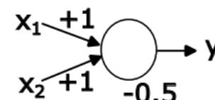
$$\begin{aligned}y &= b\text{sign}(w_0 + w_1 x_1 + w_2 x_2) \\&= b\text{sign}(-0.5 + x_1 + x_2)\end{aligned}$$
