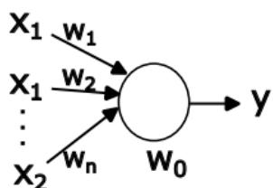
$$\begin{aligned}\xi &= \vec{w} \cdot \vec{x}^T = \sum_{i=0}^n w_i x_i \\ &= w_0 + \sum_{i=1}^n w_i x_i\end{aligned}$$
